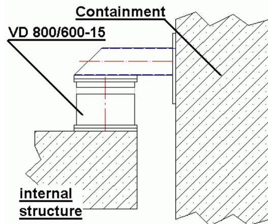
Fig. 11. Sketch of dampers' installation
