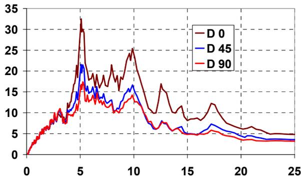
Fig. 12. Response Spectra at the upper deck of the reactor island. Rock base
