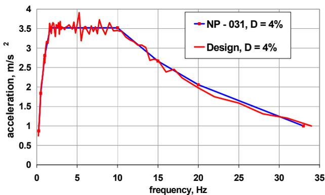
Fig. 3. Designed and standard response spectra (damping 4%) [1]
