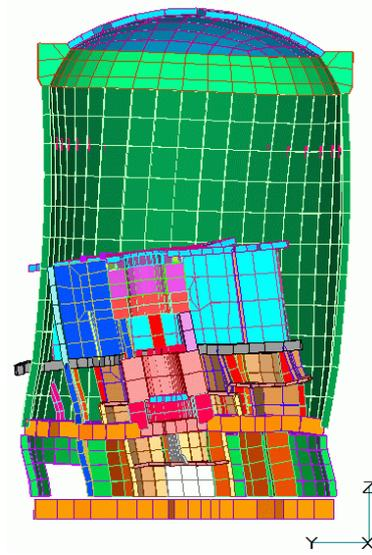
Fig. 5. Natural mode shape. Frequency 5.20Hz.
