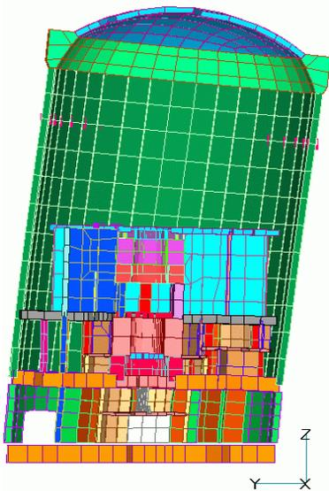
Fig. 4. Natural mode shape. Frequency 3.07Hz.
