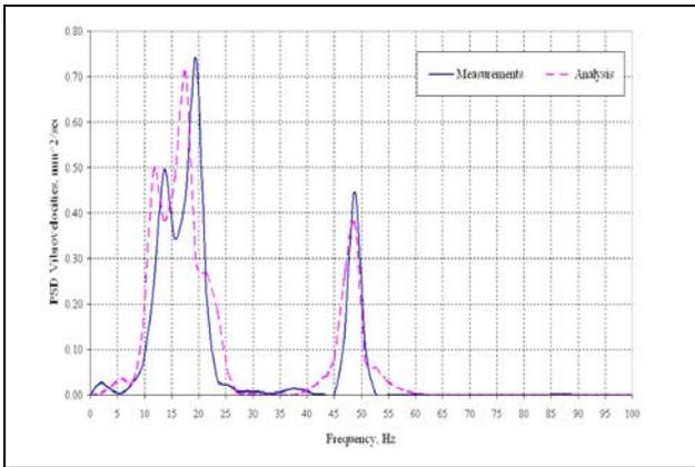
**Figure 2.** Comparison of Measured Experimentally and Analytical PSD Vibrovelocity (Eigen Value Analysis) for Measurement Point 1 (Valve 1234 Body).
