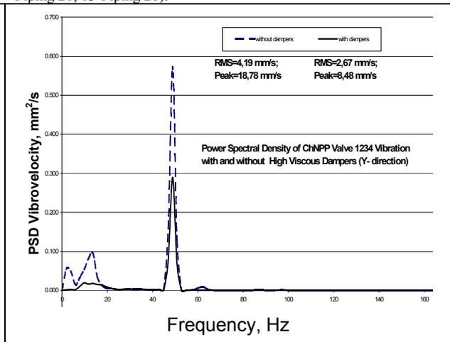
**Figure 5.** Vibrovelocity PSD before and after Damper Installation. Valve 1234, Measurement Point 1, Direction Y.
