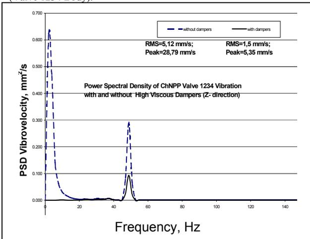
**Figure 4.** Vibrovelocity PSD before and after Damper Installation. Valve 1234, Measurement Point 1, direction Z.
