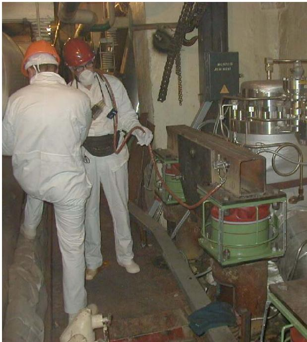
**Figure 8.** Vibration Measurements on the Valve's 1211 Damper Plate.
