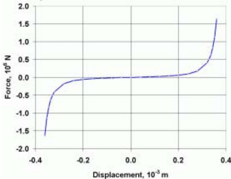
Fig. 12 Thrust Bearing Reaction vs. Rotor Displacement
