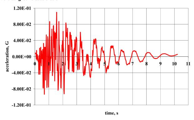
It should be noted that input motion is given by time history acceleration with duration of 10.22 s and time step 0.02 s.
