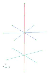
Steam generators are modeled by "shell" elements. To represent inertial characteristics of the steam generator its mass is distributed on the surface of "shell" elements. Vertical steam generator supports are modeled as vertical springs by the "directional spring" elements. Horizontal steam generator supports are hydraulic snubbers modeled by "axial spring" elements.
